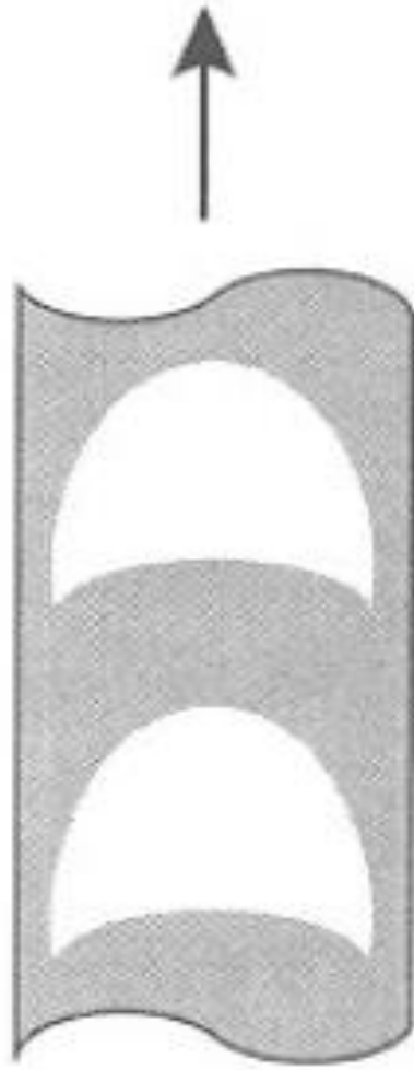
Slug flow (gas pockets)
