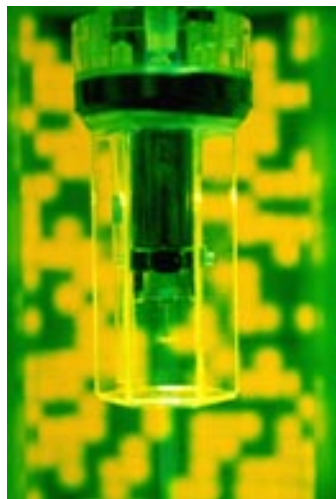
Fig. left: Respirometry chamber to measure flight forces and metabolic rates in the fruit fly Drosophila . Fig. right: 'Virtual reality' - flight simulator for insects
