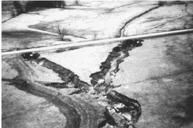
Fig. 10. Oblique aerial photograph of widening caused by channel incision in the neighbouring Johnson Creek, Panola County, MS, USA. Flow is towards the camera. Channel incision is not obscured by riparian vegetation but has been arrested by bridge crossings (middle photograph). Comparison with the channel above the bridge shows the incised cross-sections to be considerably wider and deeper (Photographer: unknown).
