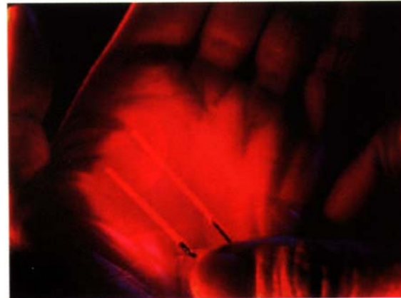
Figure 5. Light Emitting Diode (LED) sources for clinical PDT. (a) array for skin lesion treatments (courtesy EXFO Inc, Canada), (b) small array for intra-oral application (courtesy PRP Optoelectronics, England), (c) interstitial linear arrays (courtesy Light Sciences Inc., USA).
