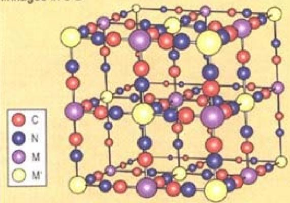
When M = Cr, M' = Ni material is a ferromagnet,  $T_c = 90K$ When M = V, M' = Mn material is a ferrimagnet,  $T_c = 125K$ When M = Cr, M' = V material is a ferrimagnet,  $T_c = 315K$
