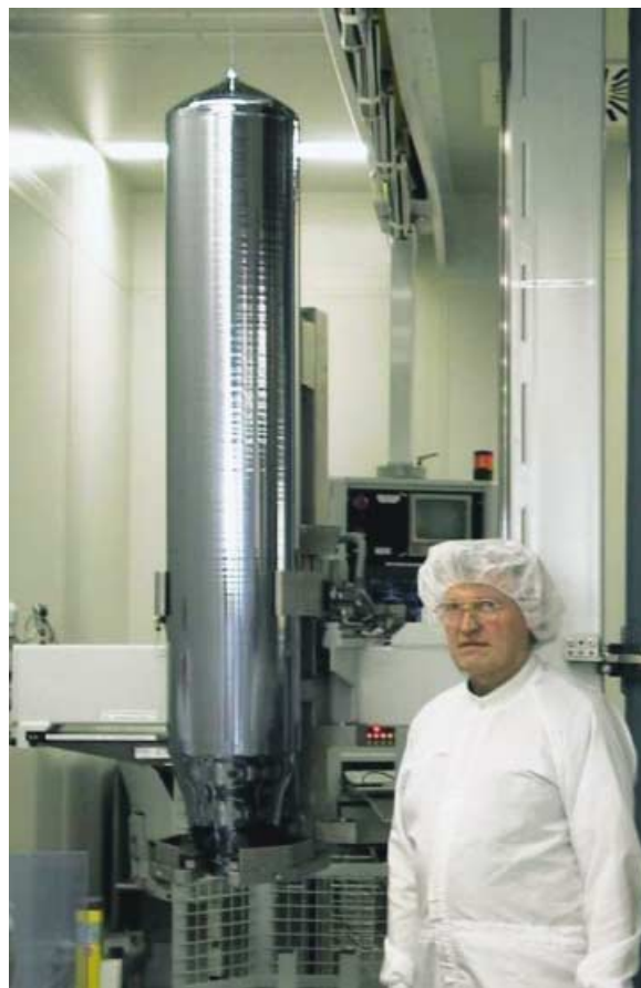
Figure 5. A single crystal of silicon, 300 mm in diameter, 2 m long, and weighing 265 kg, drawn using the CZ process. (Photograph: Wacker-Chemie).
