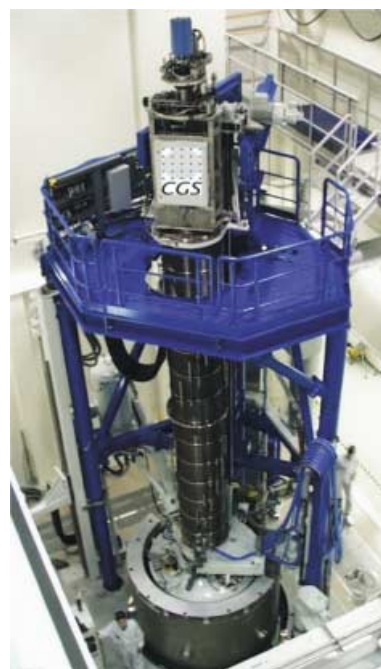
Figure 8. CZ crystal drawing apparatus for crucible diameters of up to 102 cm and a maximum of 600 kg silicon melt. [35] (Photograph with kind permission of Crystal Growing Systems GmbH).
