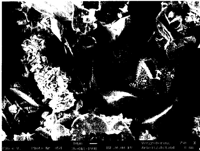
Fig. 11: Simultaneous dissolution of glass (right hand side) and recrystallization to zeolite (left hand side) under hp-hydrothermal conditions.
