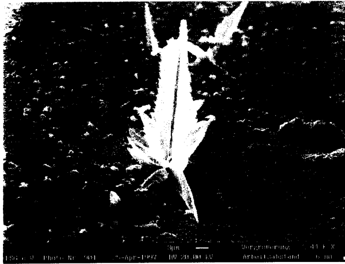
Fig. 10: First state of zeolite crystal formation by growth of nuclei on glass surface.
