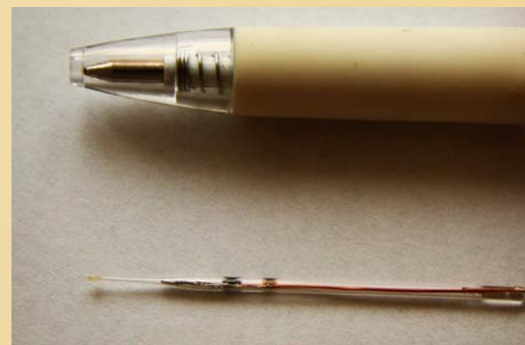
porphyritic microsensor ( 7 \mu\text{m} in diameter, typical length 0.5-1 mm)
