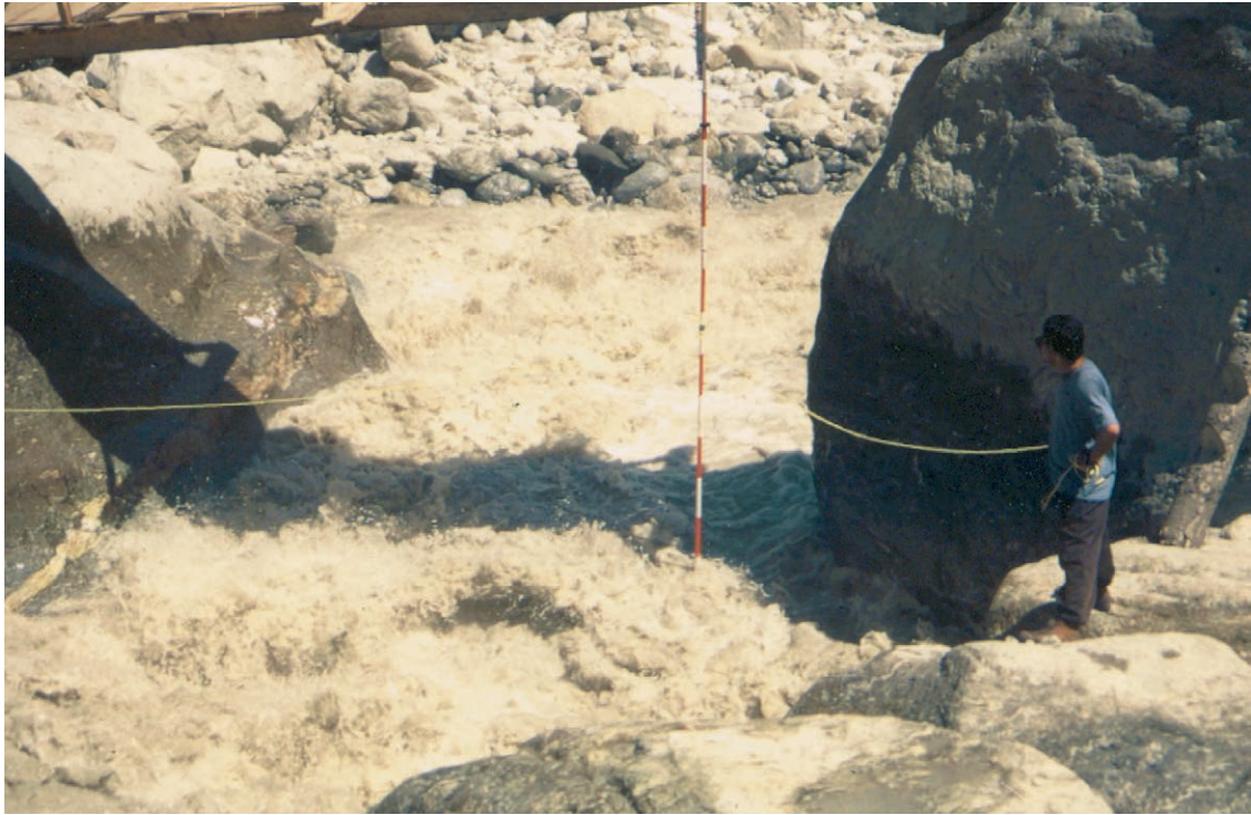
Fig. 7. Probing bedrock conditions and channel cross sections at the Raikot Bridge crossing. Guide ropes were used to stabilize the stadia rod as dynamic flow conditions prohibited direct push approaches.
