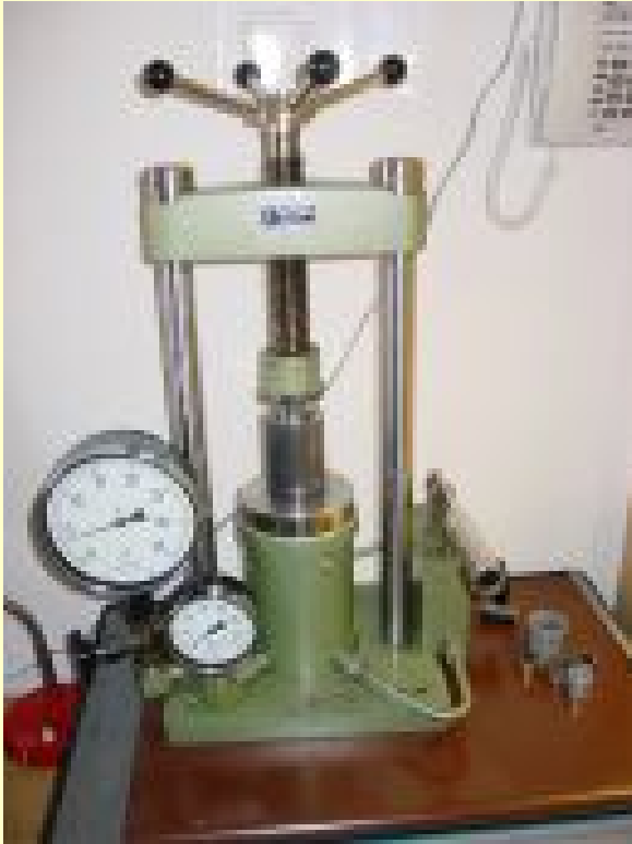
Hydraulic Uniaxial Press Maximum pressure: 120 MPa
