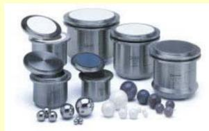
Particles repeatedly subjected to deformation, cold welding, and fracture, homogenization on an atomic scale
