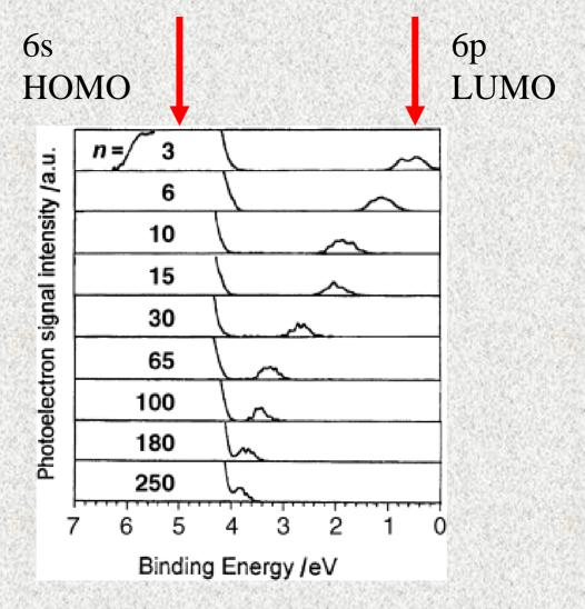
Photoelectron spectra of Hg clusters of nuclearity n The 6p peak moves gradually towards the Fermi level the band gap shrinks with increase in cluster size
