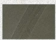
A picture of a typical multi-shell nanotube taken using TEM (Source from Dr. P. M. Ajayan)
