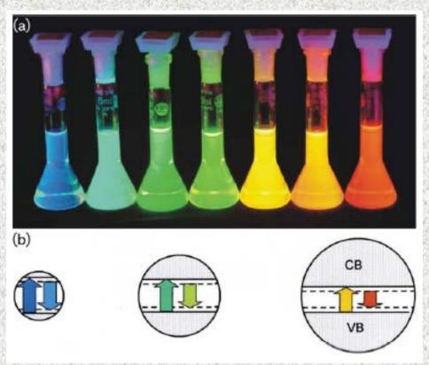
Fluorescence of CdSe–CdS core–shell nanoparticles with a diameter of 1.7 nm (blue) up to 6 nm (red), smaller particles have a wider band gap
