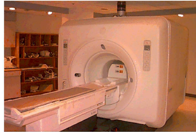
Figure 3. Magnets for (a) NMR 900 MHz, superfluid helium cooled and (b) full-body MRI, liquid helium bath cooled with active shield refrigeration (Bruker)
