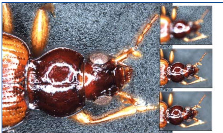
Fig. 24: The software extracts the focused areas from the component images of an image series and reassembles them into one infinitely sharp image. The example shown here is the resulting image computed automatically using 25 images of a Bembidion tetracolum sample.
