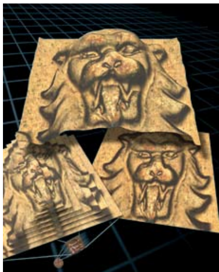
Fig. 25: This image shows how far money can go: This Singaporean coin detail was captured using a ColorView digital CCD camera and processed using the realignment, extended focus and 3-D imaging software modules. Capture and automatically align multiple component images into a high-resolution composite using the MIA module. Extract the sharpest details within the component images and reassemble into one single image having infinite depth of focus with the module EFI. Finally, create incredibly realistic views using height and texture information attained through the perspective functions of the 3D module.
