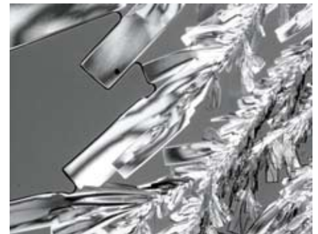
Fig. 26: Vitamin C crystals observed in polarised light.
