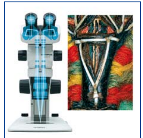
Fig. 54: The stereomicroscopic (Galileo type) light path – two microscopes in one – offers observation of specimens at the natural convergence angle of our eyes. This makes the 3D topography visible. However, when the specimen is documented the image will nevertheless remain a two-dimensional view.
