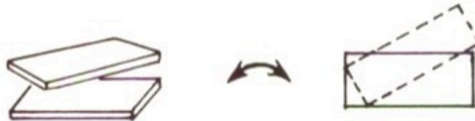
Fig. 2.17 Ways in which adjacent bases may move relative to one another (seen from two different positions).
