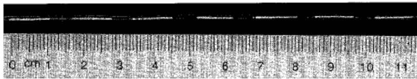
FIG. 1. High throughput flow cytometry. A : Schematic view of the flow cytometer, autosampler, and peristaltic pump. B : Adjacent samples of latex microspheres separated by air in the 0.02-in (254- \mu m) ID tubing between the peristaltic pump and the flow cytometer.
