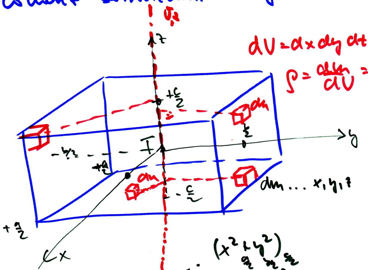
$$I_{0,z} = ? = \iiint_{V_{\text{plate}}} r^2 \rho dV = \rho \int_{-\frac{a}{2}}^{\frac{a}{2}} \int_{-\frac{b}{2}}^{\frac{b}{2}} \int_{-c}^{+c} (x^2 + y^2) dm dx dy$$
