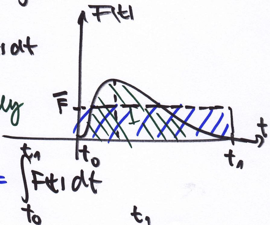
$$\bar{F} (t_1 - t_0) = \int_{t_0}^{t_1} \vec{F}(t) dt$$
