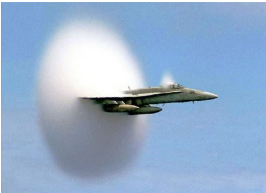
An F/A-18 Hornet photographed just as it broke the sound barrier. Credit: Ensign John Gay, USS Constellation, US Navy
