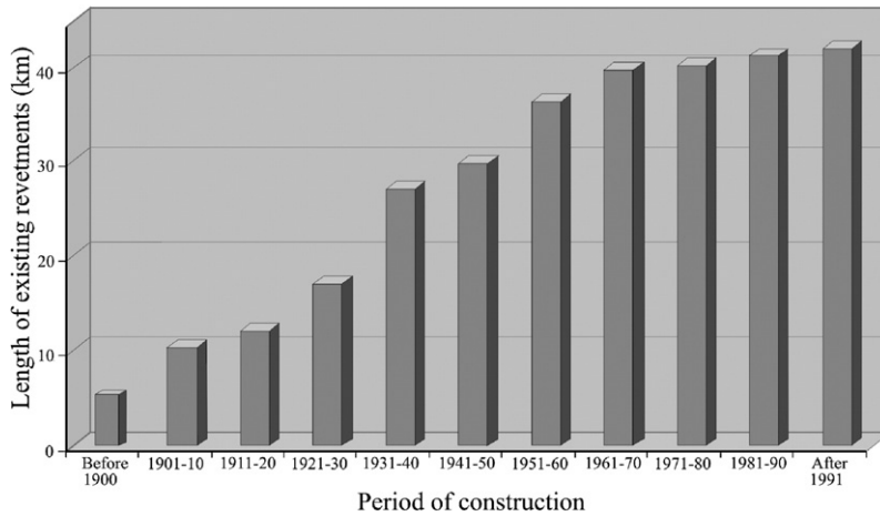
Fig. 2. Revetment constructions along the 88 km long Hungarian section of the Lower Tisza River.
