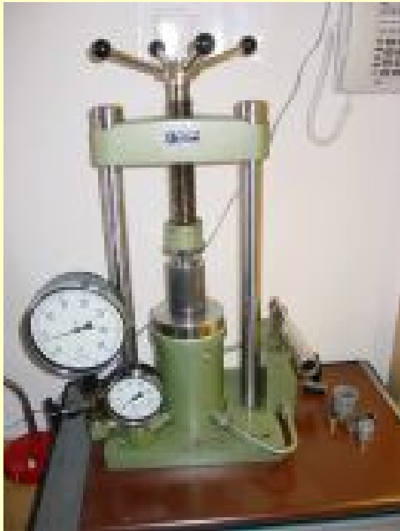
Hydraulic Uniaxial Press Maximum pressure: 120 MPa
