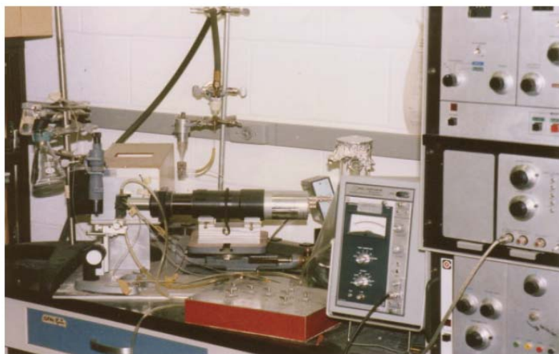
FIG. 1. The Fulwyler instrument as installed in Dr. Boris Rotman's Laboratory in Brown University, immediately prior to disassembly in March 2005. The instrument had not been altered or moved since installation in 1967, except for the addition of a laser instead of the UV lamp.
