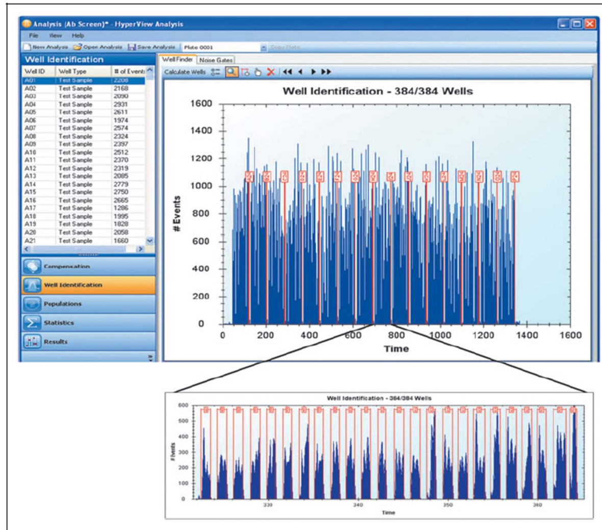
Fig. 4. Screenshot from HyperView showing an example of the Well Identification process. Data from the 384-well plate is collected in to a single flow cytometry standard file, which is shown in the main window. The data are deconvolved by the software algorithm to identify each peak with a well address on the plate. One row is expanded to show temporally spaced individual peaks.
