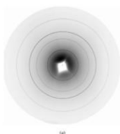
Figure 3 a) The X-ray pattern of Zn(OHPO_4) in a suspended mixture with water. The sharp peaks of the beam stop is visible in the center of the diffraction image. b) The X-ray diffraction curve of Zn(OHPO_4) in a suspended mixture with water.
