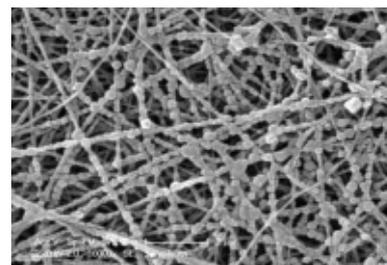
Nanoparticles of titanium dioxide anchored on polyurethane nanofibres
