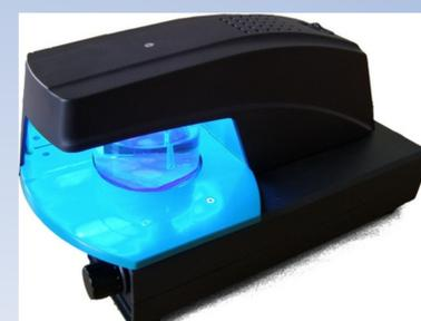
Another testing device developed by NANOPIN is the **chamber for testing self-cleaning and antimicrobial properties of active films and coatings**. The box has transparent front wall with two glow ports for sampling, inside of the chamber are jets for producing fine liquid sprays, electricity cut-outs and the vent of the ventilation fan are at the rear wall of the chamber. At the chamber cover the illumination system of 4 UV black-light lamps is mounted (Osram UVA 350 to 400 nm, L 18 W/73).
