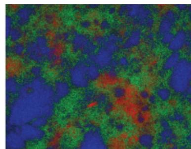
Surface (95 x 75 micrometres) of self-cleaning paint based on novel nanocomposite photocatalyst scanned by Energy Dispersive X-ray (EDX) spectroscopy for present elements (titanium - green, silicon - red, calcium - blue)
