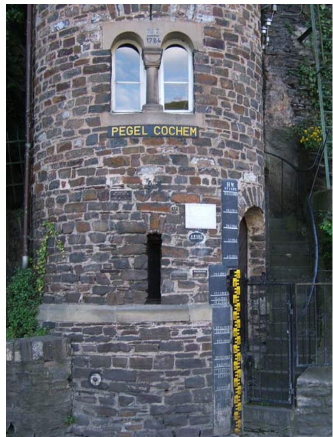
Fig. 16 Epigraphic marking illustrating the water level of 28 February 1784 (above the window of the Cochem water gauge on the River Mosel, significantly exceeding all other recorded events; photo Jiří Štrupl)
