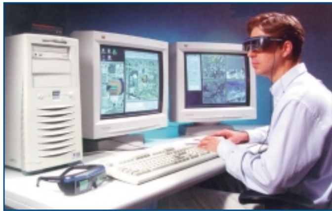
An LH Systems DPW with twin screens running the SOCET SET software under Windows NT on a Dell PC. The operator is utilizing a 3D hand controller to control the position of the measuring mark and is viewing the stereo-model in 3D with the new lower-cost CrystalEyes wired spectacles from StereoGraphics. (Courtesy LH Systems)
