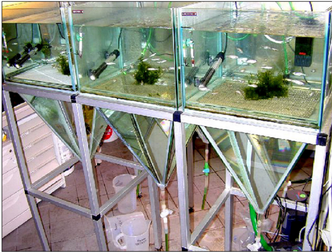
Fig. 5: Setup of the tanks used for breeding zebrafish in the Berlin laboratory (Leibniz-Institute of Freshwater Ecology and Inland Fisheries): Large groups of zebrafish are maintained in tanks the bottom of which has been replaced by a stainless steel grid to avoid predation of the eggs by the parent fish. The tanks are sitting on a big funnel, which allows simple release of the newly spawned eggs (courtesy of Dr. T. Meinelt, IGB).
