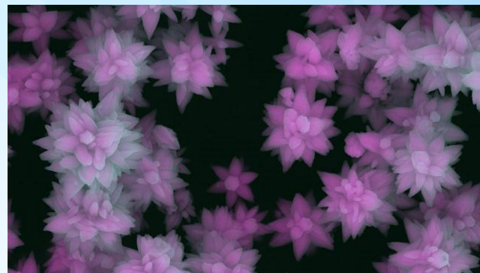
Zno nanoparticles obtained by hydrothermal synthesis using microwave heating
