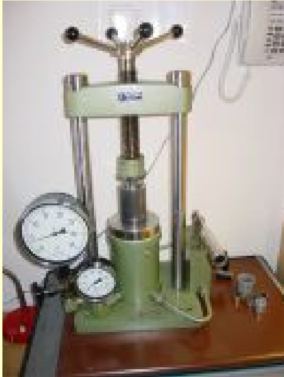
Hydraulic Uniaxial Press Maximum pressure: 120 MPa
