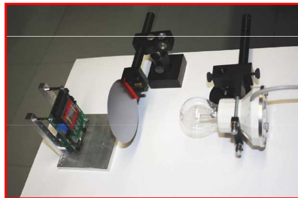
64x64 pixel IR sensor with integrated Ge photodiodes
