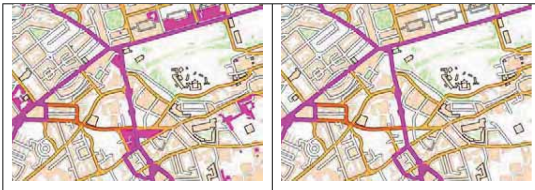
Figure 91: Buildings intersecting with the roads are eliminated (shown in pink, left); result after elimination (right).
