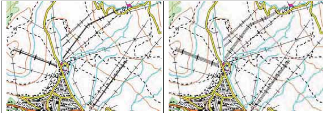
Figure 89: Ski-lifts before (left) and after (right) displacement with PUSH - specially look at the ski-lifts.
