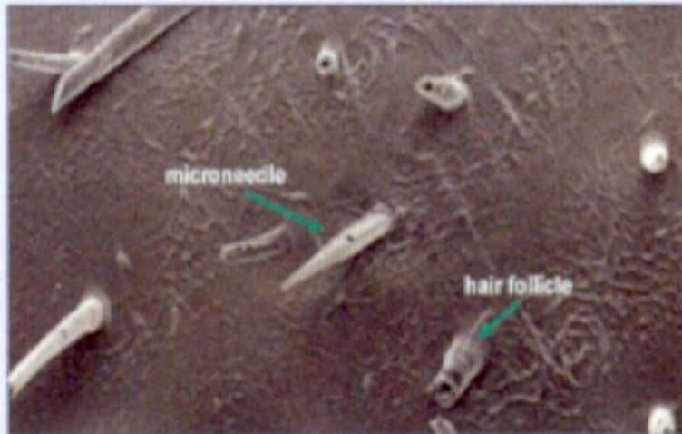
Figure 1. Microneedle penetrating swine dermis. ( Electron microscopy by H. Sugg, BD Technologies )
