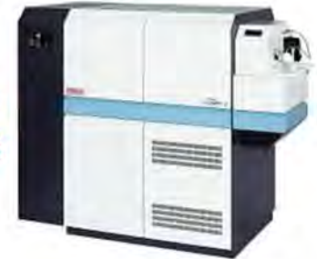
Thermo Finnigan Element2 ICP-MS
