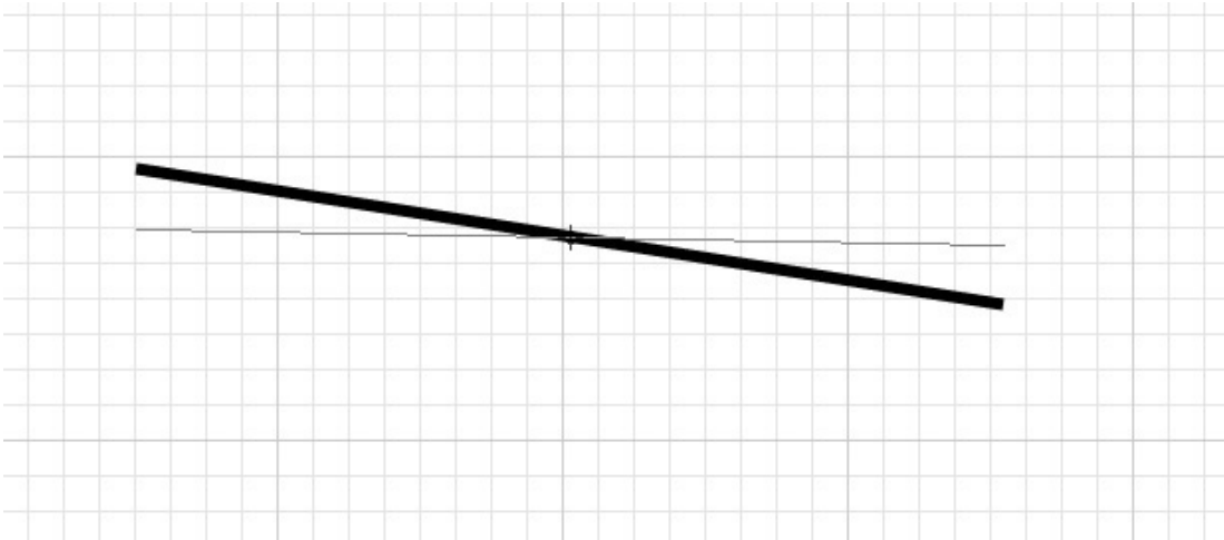
Fig. 9: Scalebars are drawn with the Pencil tool. Both ends of the scalebar are marked. After a rightclick with the mouse, select grouping and "R" for Rotate, then align the scalebar using the mouse.
