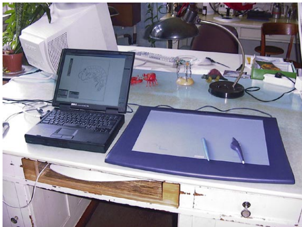
Fig. 1: Setup of digital drawing equipment. On the left a notebook computer, on the right a WACOM digitiser board with two different pens.
