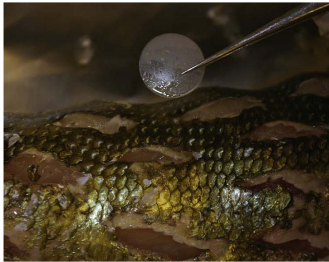
Fig. 1. Circular PDMS thin-films were inserted into intact fish tissue for equilibrium sampling of PCBs. The samplers were retrieved after time periods of 1 h up to 7 d. Picture: U. Berger.
