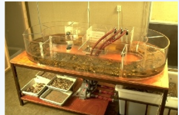
Figure 7. Principal components of a standardized aquatic indoor microcosm, based on an artificial medium with 10 species of primary producers and 5 species of grazers. From Taub (44), with permission.
