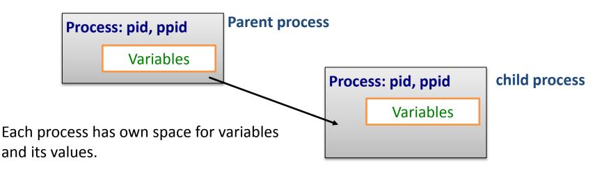
Child process when started gets **copy** of **exported** variables and its values from parent process. These variables can be changed by any way or remove them and new variables can be defined too. **All these changes are not visible to original variables in parent process and are deleted when child process finishes.**
