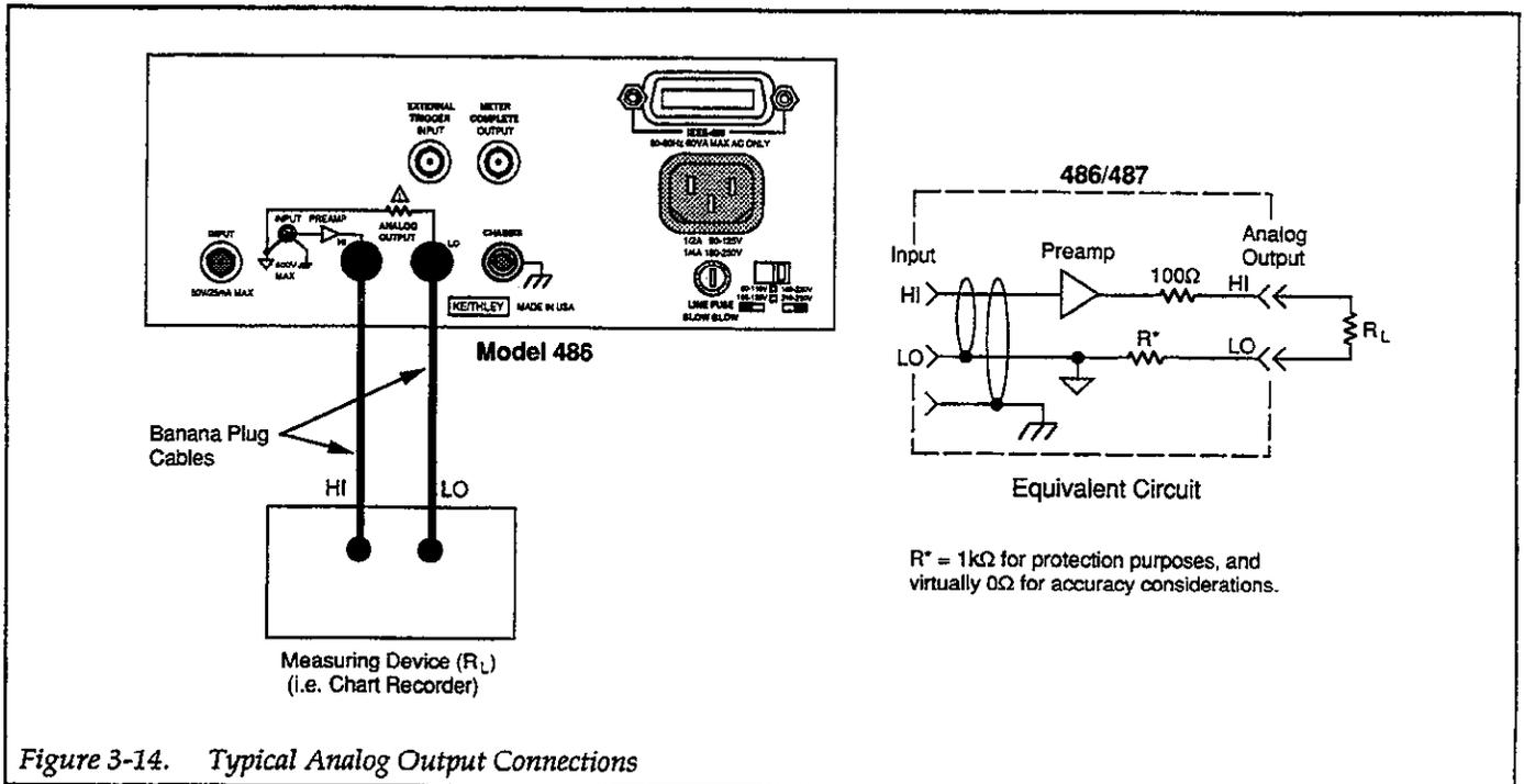
Figure 3-14. Typical Analog Output Connections
