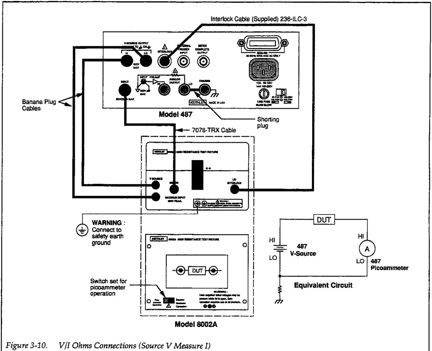
To make V/I ohms measurements, the Model 487 is configured to source voltage and measure current (Source V Measure I). The V/I feature simply performs the calculation ( $R = V/I$ ) and displays the resistance reading in ohms. The results of any source V measure I test can be converted to resistance by using the V/I ohms function. Paragraph 3.15 expands on tests that source voltage and measure current, and provides some examples that are particularly applicable to the V/I ohms function.
