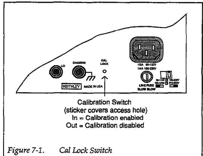
Figure 7-1. Cal Lock Switch
