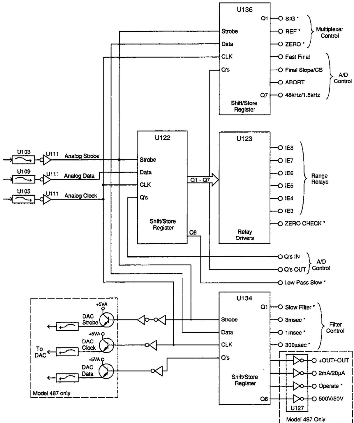
Figure 6-10. Analog Control Circuitry
