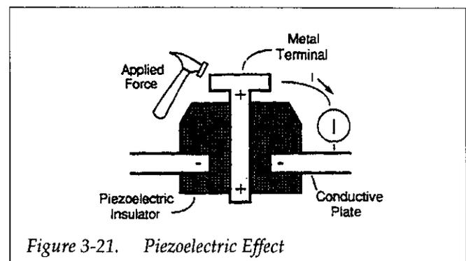
To minimize the current due to this effect, it is important to remove mechanical stresses from the insulator and use insulating materials which have minimal piezoelectric effects, such as sapphire, Teflon®, or PVC.
