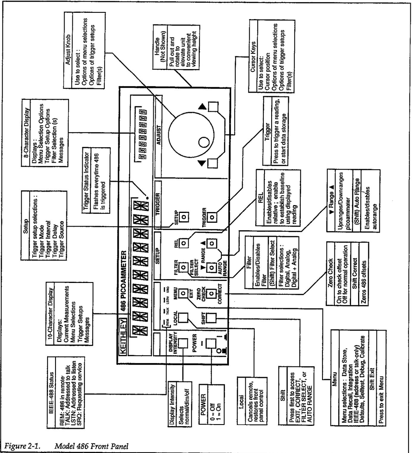
Figure 2-1. Model 486 Front Panel
