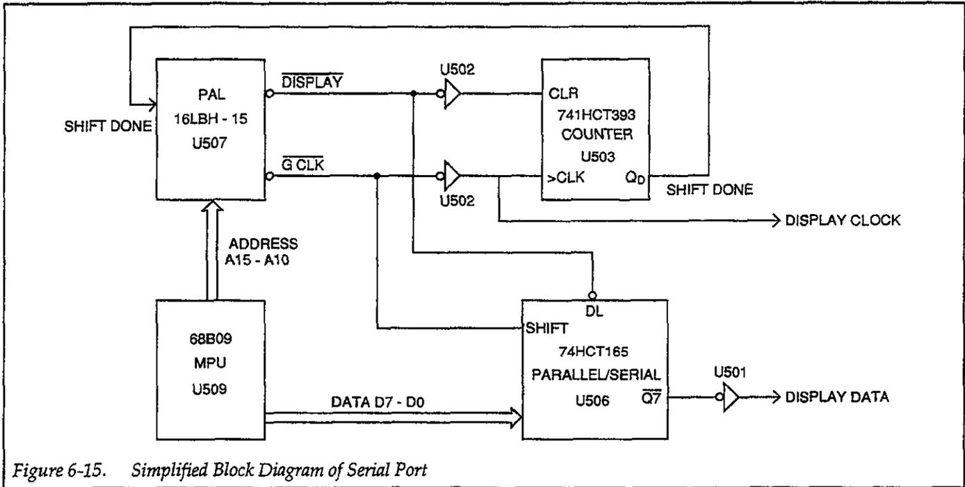
Figure 6-15. Simplified Block Diagram of Serial Port
