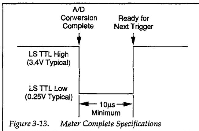
Figure 3-13. Meter Complete Specifications
