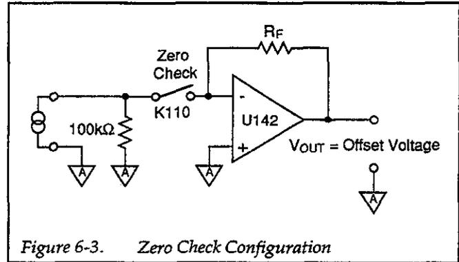
Figure 6-3. Zero Check Configuration
