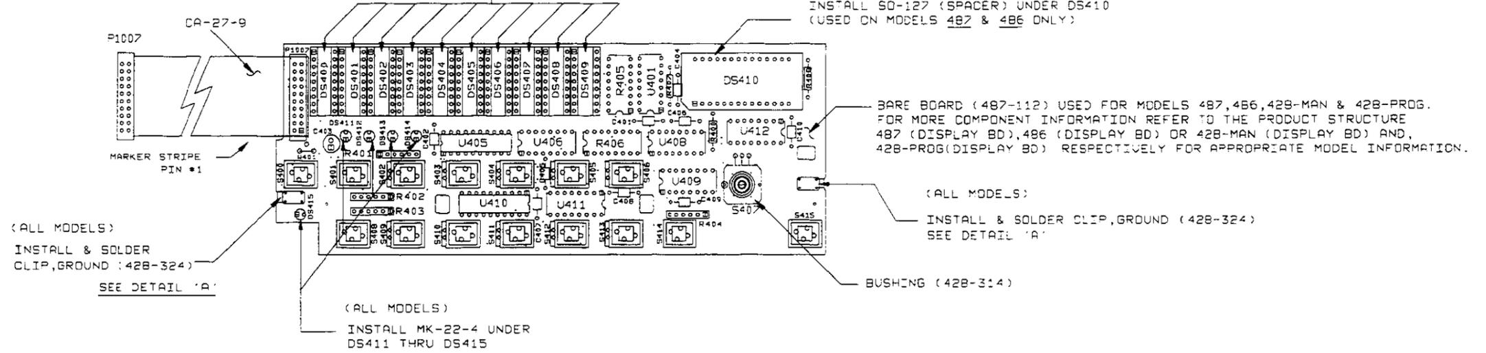
BARE BOARD (487-112) USED FOR MODELS 487, 486, 428-MAN & 428-PROG. FOR MORE COMPONENT INFORMATION REFER TO THE PRODUCT STRUCTURE 487 (DISPLAY BD), 486 (DISPLAY BD) OR 428-MAN (DISPLAY BD) AND, 428-PROG (DISPLAY BD) RESPECTIVELY FOR APPROPRIATE MODEL INFORMATION.
