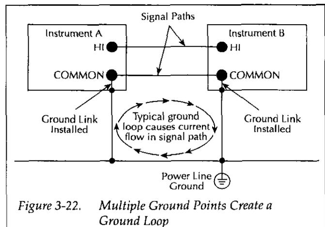
Figure 3-22. Multiple Ground Points Create a Ground Loop
