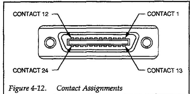
Figure 4-12. Contact Assignments
