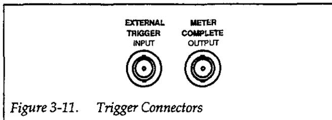
Figure 3-11. Trigger Connectors
