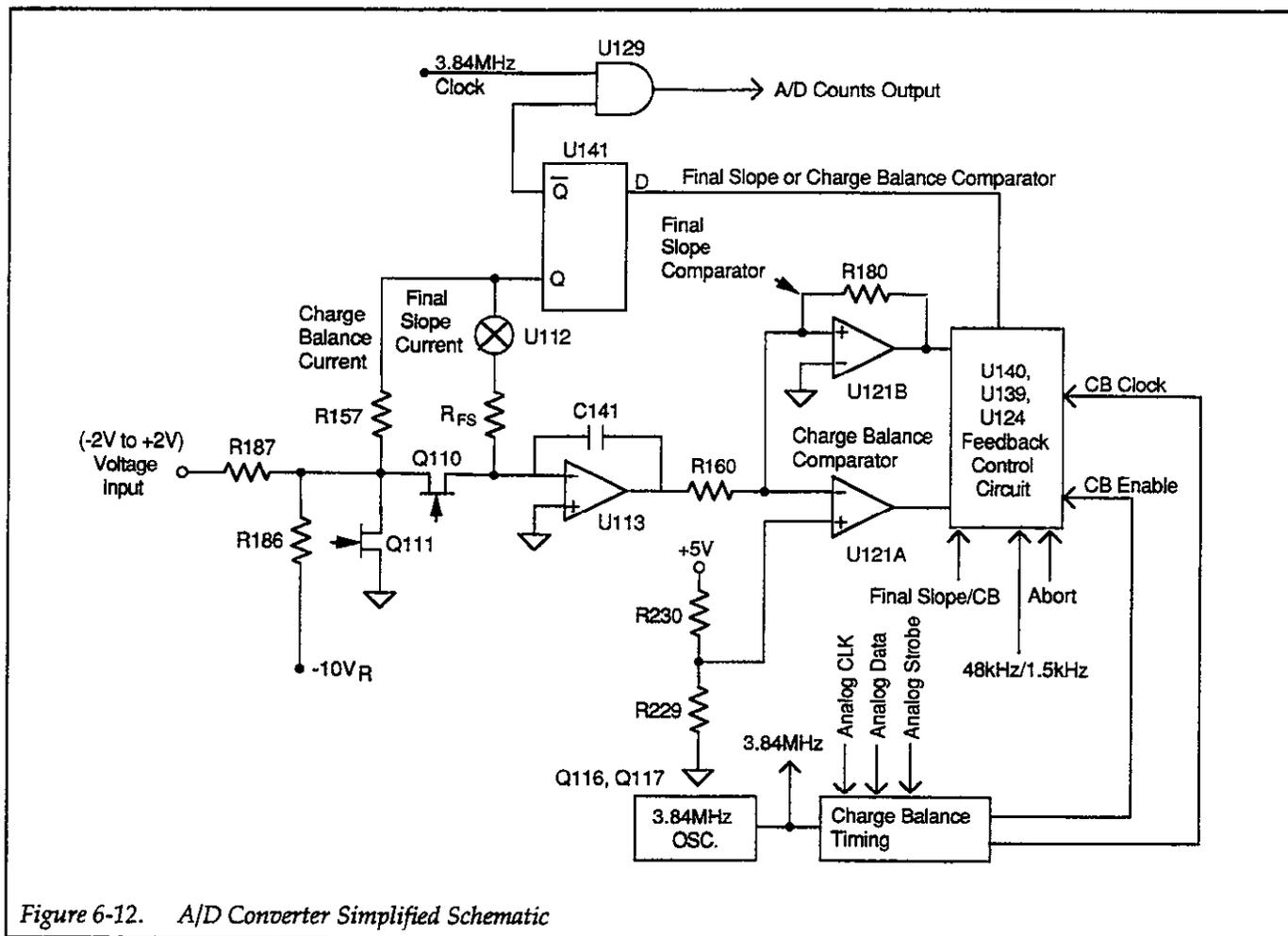
Figure 6-12. A/D Converter Simplified Schematic
