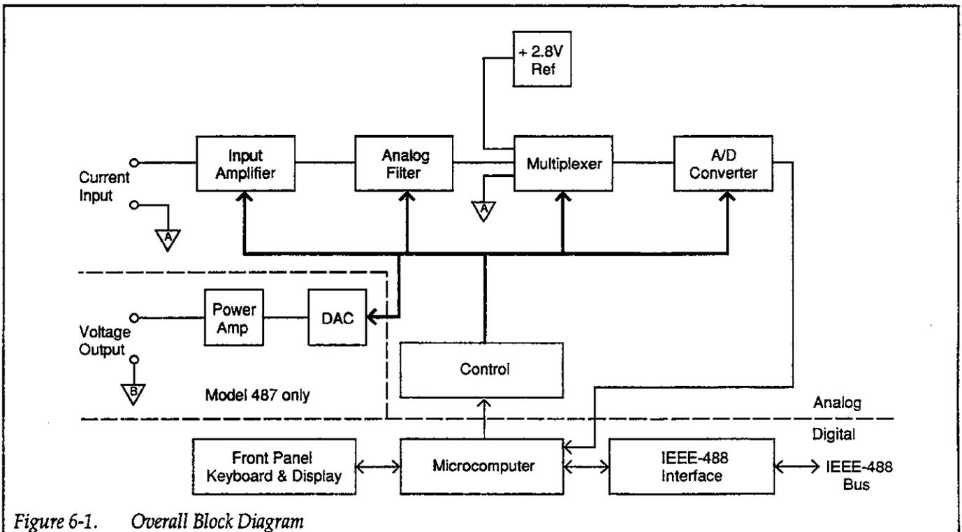
Figure 6-1. Overall Block Diagram
