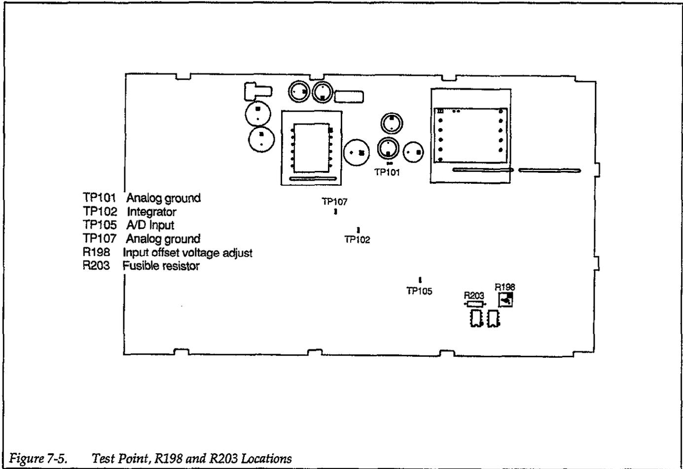
Figure 7-5. Test Point, R198 and R203 Locations
