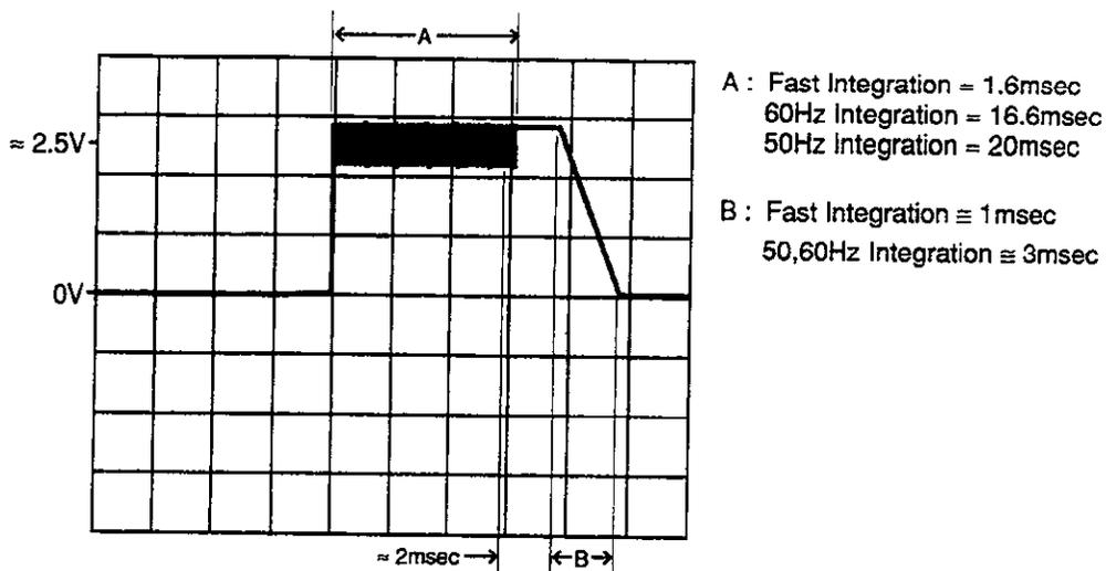
Figure 7-6. Integrator Output (Typical)
