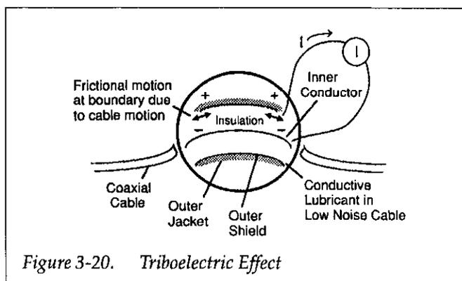
"Low-noise" cable greatly reduces this effect. It typically uses an inner insulator of polyethylene coated with graphite underneath the outer shield. The graphite provides lubrication and a conducting equipotential
