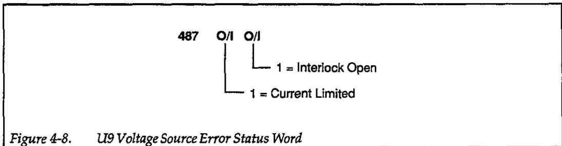
Figure 4-8. U9 Voltage Source Error Status Word
