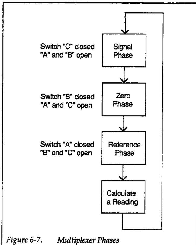
Figure 6-7. Multiplexer Phases
