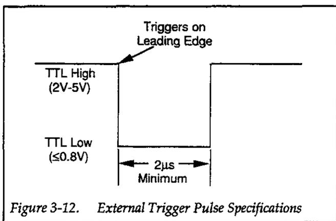
Figure 3-12. External Trigger Pulse Specifications
