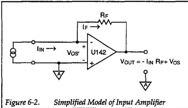
Figure 6-2. Simplified Model of Input Amplifier
