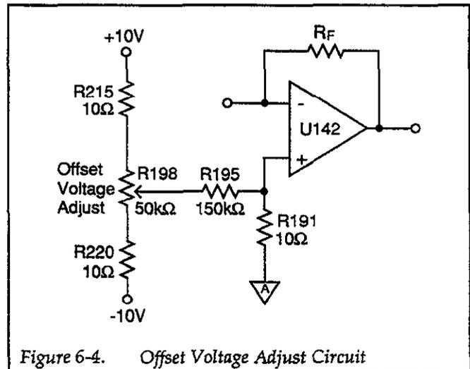
Figure 6-4. Offset Voltage Adjust Circuit
