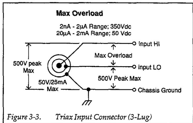
Figure 3-3. Triax Input Connector (3-Lug)
