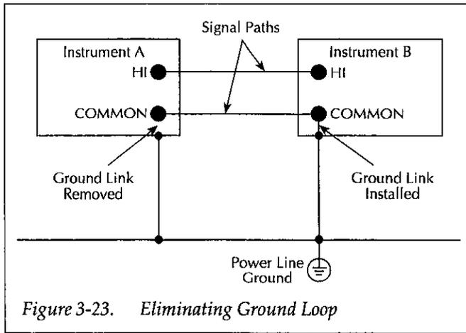
Figure 3-23. Eliminating Ground Loop
