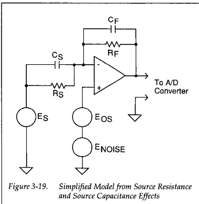
Figure 3-19. Simplified Model from Source Resistance and Source Capacitance Effects
