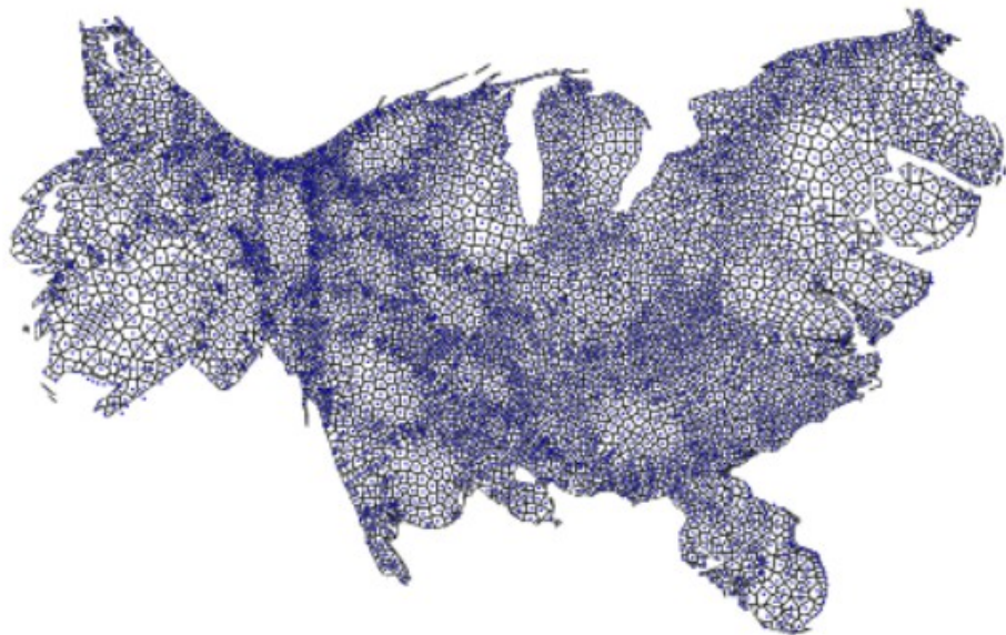
FIG. 3: Near-optimal facility location on (a) a cartogram equalizing the population density \rho and (b) a cartogram equalizing \rho^{2/3} .
