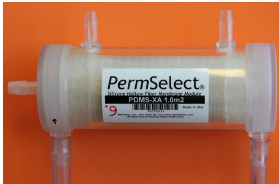
Fig. 1. The passive dosing unit showing the inlet (lower left) and outlet (lower right) ports for the perfusion of the lumen. The other three ports are for the perfusion of the shell space.
