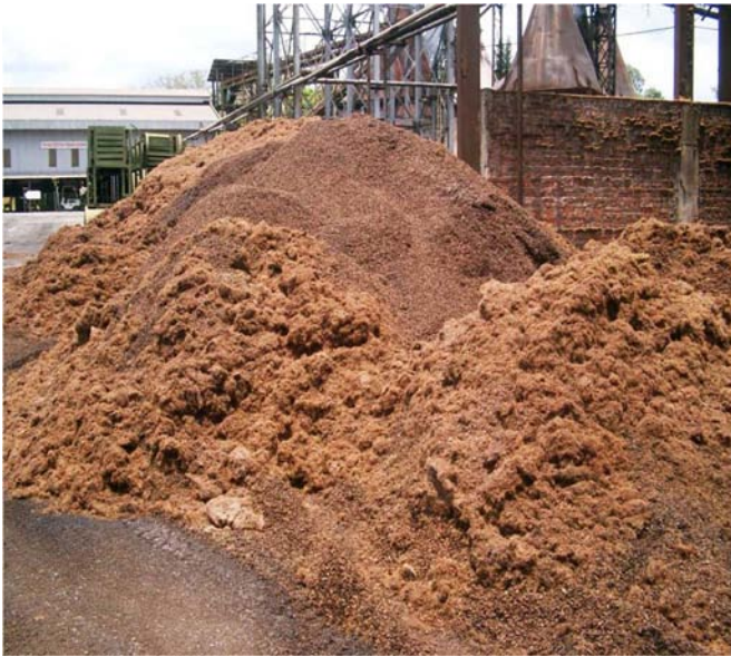
Picture 5: Residue from palm oil extraction, partly used for power generation. Photograph: IFEU
