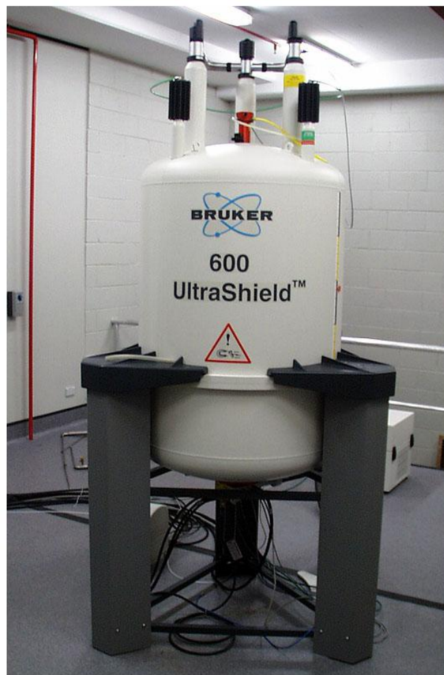
600 MHz Ultrashield NMR Spectrometer
