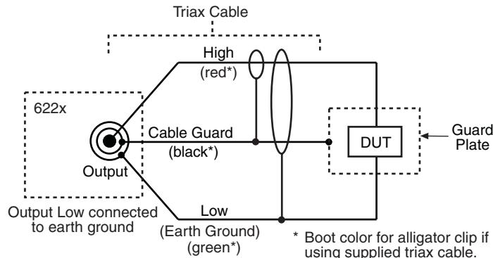
A safety shield must be used whenever hazardous voltages (>30Vrms, 42Vpeak) will be present in the test circuit. [Figure 2-10](#) shows how to make guarded connections with the use of a safety shield.
