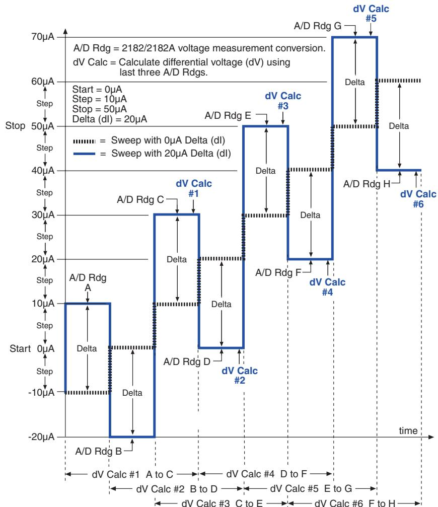
**dV Calculations** – The following equations are used by the 622x to calculate differential voltage (dV). To calculate dV, points A through H are 2182/2182A voltage measurements (A/D readings).
