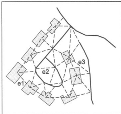
Fig. 25. Local Delaunay triangulation between buildings and adjacent roads (after Ruas 1995). Edge e_1 denotes an edge connecting two buildings; e_2 connects two vertices on a road; and e_3 connects a building and a road.
