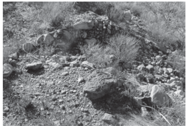
Figure 5.31 View of survey tape laid out along a segment of the crest of the 1887 scarp at the Dos Escarpas site. Instead of being straight, the white tape has a sinuosity of 1.4.
