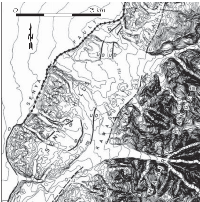
Figure 3.13 Characteristics of thrust faulted mountain fronts in Japan. A. Contour map (interval 10 m) of the Senya Hills piedmont foreland of the Mahiru Range, in northern Honshu Island draining to the Sea of Japan. The Kawaguchi thrust fault (dashed line) bounds the internal front. The dotted line along the range-bounding Senya thrust fault indicates the surface rupture of the 1896 Rikuu earthquake. From Figure 4 of Ikeda, 1983.
