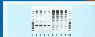
Fig. 2. Typical separation in the Model 111 Mini IEF Cell (5% polyacrylamide gel with 2% Bio-Lyte 3/10 ampholytes). Focusing was carried out in a stepped fashion (100 V for 15 minutes, 200 V for 15 minutes, 450 V for 1 hour). Samples are: lanes 1 & 10: Bio-Rad's IEF Standards; lanes 2-5: Dilutions of horseradish peroxidase; lanes 6-9: Dilutions of Japanese water moccasin snake venom.
