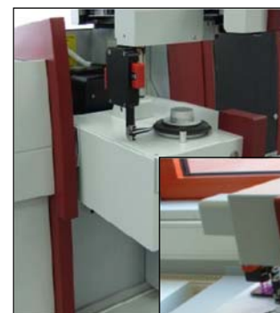
New robotized sample introduction system SSA 600 with integrated sampler for chemical sample modification
