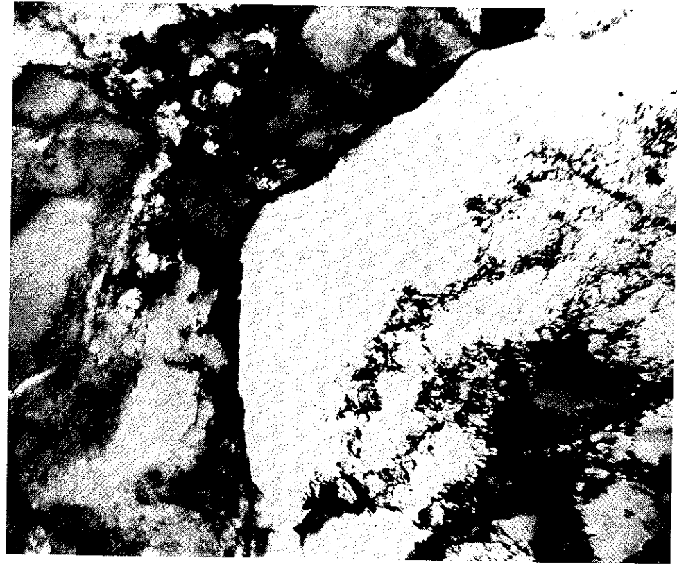
Fig. 3.26 Grain boundary migration in nickel pulled 10% and annealed 10 min at 425 °C. The region behind the advancing boundary is dislocation-free. (After J. Bailey and P. Hirsch, Proceedings of the Royal Society, London, A267 (1962) 11.)
