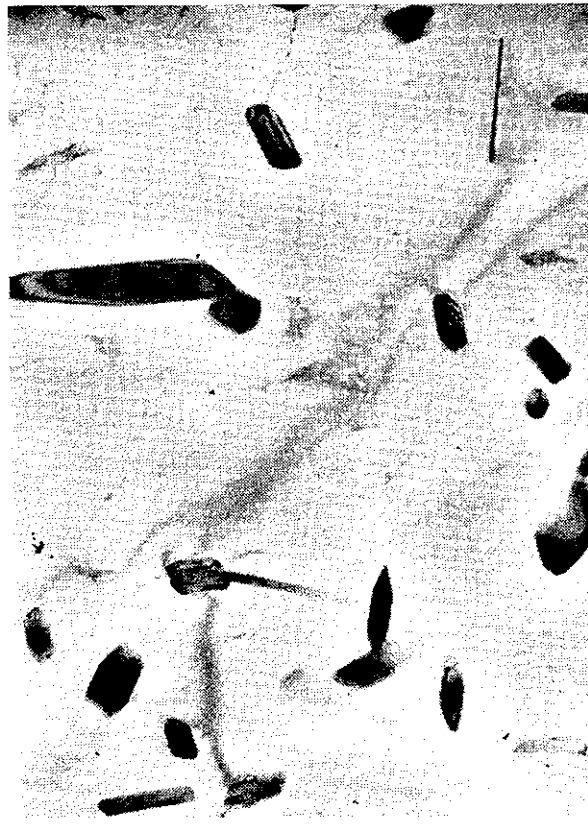
Fig. 3.44 Electron micrograph showing incoherent particles of \theta in an Al-Cu alloy. (After G.A. Chadwick, Metallography of Phase Transformations , Butterworths, London, 1972, from C. Laird.)
